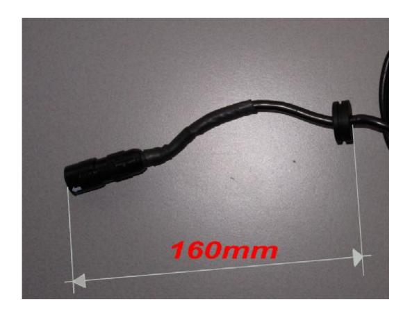
ü In order to guarantee the water pollution, insert 2 pipe rubber grommets at the extremities of the plastic tube of 6 mm diameter, as illustrated in the photos below.
