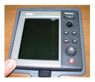
Insert the suncover as illustrated, rotating up to insert it in its seat.
