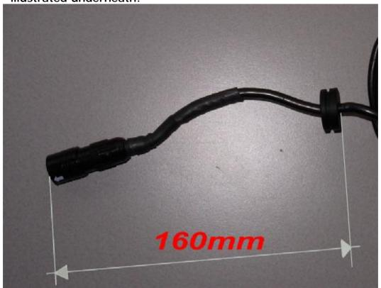
ü In case of use the power and fish finder cable (product code P1017970), use the cable rubber grommet with hole diameter 5.9mm and make a radial cut on it in order to run the cable through the rubber. See photos below.
