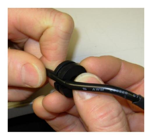
Slide the cable rubber grommet along the power cable for 160 mm, as illustrated underneath.
