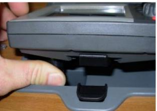
Line up the upper side of the plotter with the upper rest of the cradle.
