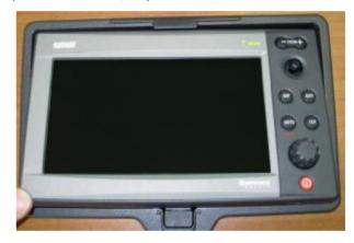
Insert the suncover as illustrated, rotating until it locks into position.
